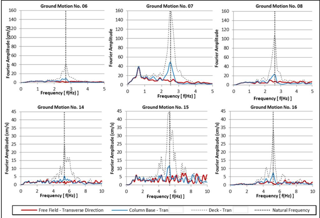
Figure 5. Fourier Spectra corresponding to each ground motion for Via California bridge (top) and Lake Crowley bridge (bottom).
