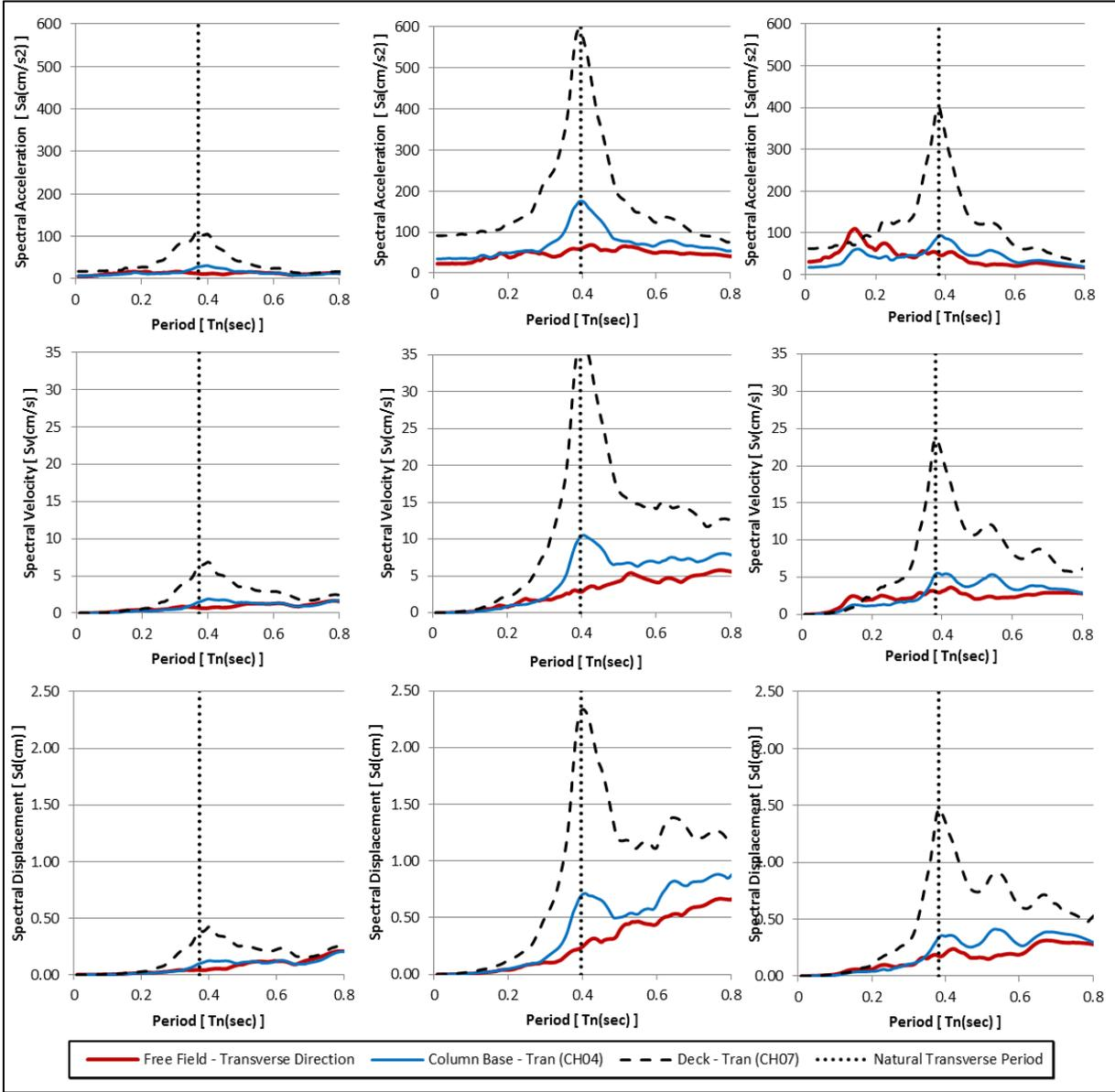
Figure 2. Response spectra for Via California Bridge corresponding to ground motions No. 06 (left), No. 07 (center) and No. 08 (right).
