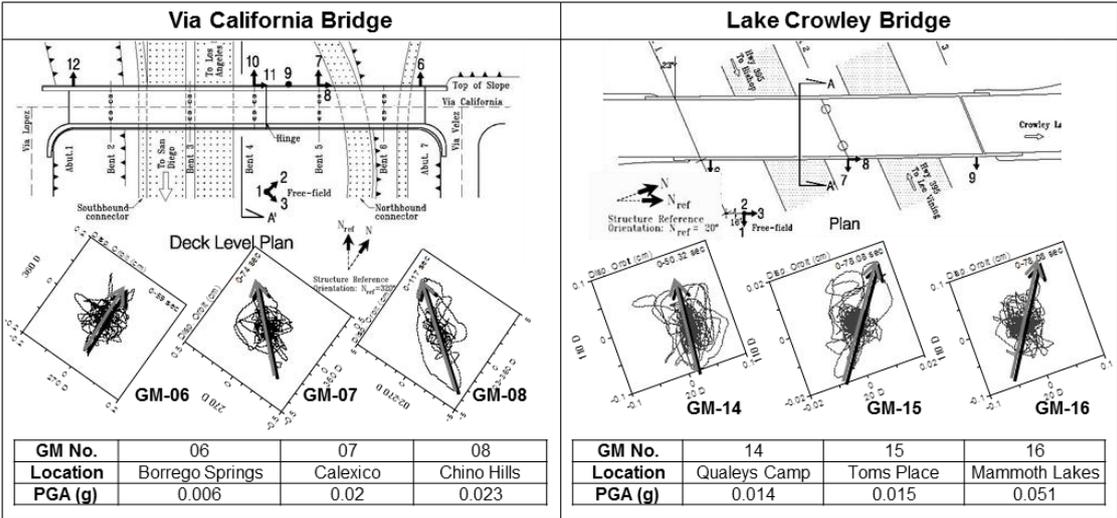
Figure 4. Estimated directionality of ground shakings and incidence to analyzed bridges.
