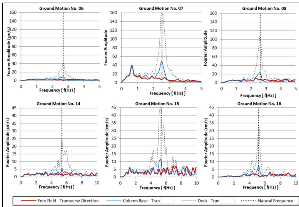
Figure 5. Fourier Spectra corresponding to each ground motion for Via California bridge (top) and Lake Crowley bridge (bottom).
