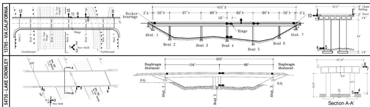
Figure 1. Summarized drawings of Via California and Lake Crowley Hwy 395 bridges
