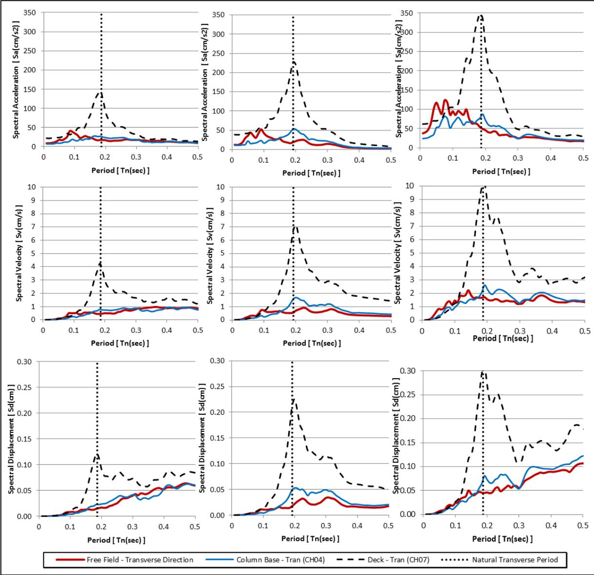
**Figure 3.** Response spectra for Lake Crowley Bridge corresponding to ground motions No. 14 (left), No. 15 (center) and No. 16 (right).
